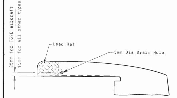
Fig 1 View on underside of Port Elevator. Stbd similar
